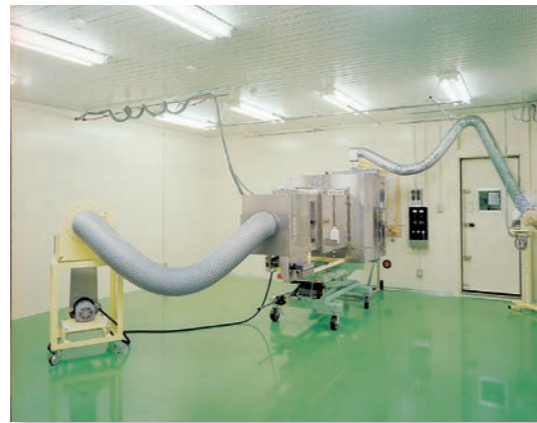
風量測定装置 Air-flow Measuring Apparatus
