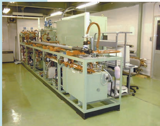
RAC用銅管(単管)熱交性能試験装置 RAC Copper-pipe (Single-pipe) Heat Exchanger Performance Testing Device
