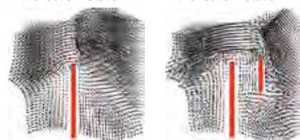
標準大型広幅断面 Cross section of standard large wide blade MR205 二重翼断面 Cross section of double-blade structure of MR205 Impeller
